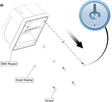
Attach EMV Reader to bracket using the hardware provided for the reader.
