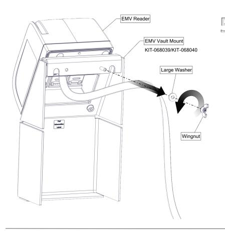
Remove wingnut and larger washer provided on bracket. This will be used in the next assembly.
