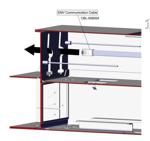
Insert cable through coin drop opening from inside machine so that the connector is on the outside. It does not matter which end is used as they are the same.
