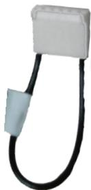
Locate the **Reader-Present / Serial Jumper** that was supplied and install it on the control board. On most control boards the connector is labeled H8.
