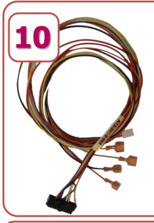
Route the main interface harness through the top of the service door, so that the card-reader connector comes through the coin-vault opening of the meter case. Make sure you have slack to work with.
