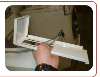
Rest the Side Car bottom on top of the meter case and slide it rearward until the curved lip securely grabs the upper-front edge of the meter case. Bolt the Side Car bottom to the new service door lid with the two (2) 1/4-20x1/2 Zinc Plated Hex Bolts and washers that were supplied with the kit.
