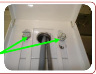
Locate the top cover of the Side Car Kit, and turn it over. Insert the WaveReader into the cover and position as shown.
