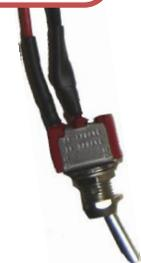
Flipping the switch will engage/disengage service mode on the machine.
