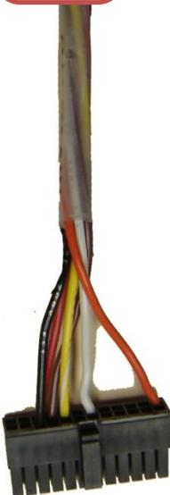
Attach the **J3 (Black) connector** into the mating connector on the back of the WaveReader Board as shown.
