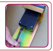
Insert the reader and bracket assembly into the coin vault opening. The mounting studs on the rear of the bracket should mate with the mounting holes at the rear of the meter case.
