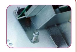
Attach the card reader cable to the card reader as shown. The locking tab on the harness connector should be aligned with the small protrusion on top of the reader connector. Press the connector in place until the tab locks.
